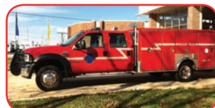
2006 EVI / Ford F-550 Light Rescue International 6.0 Diesel Engine Automatic Transmission 2 - 12 Volt 500 Watt Scene Lights Whelen LED Lightbar Brush Guard with Winch
