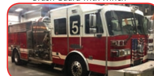
2006 Sutphen Rescue Pumper w/ CAFS Cummins ISM, Allison EVS4000 Hale 1750 GPM Top-Mount Pump 500 Gallon Poly Tank, Hale CAF System Onan 8KW Hydraulic Generator Adjustable Shelves and Slide-Out Trays
