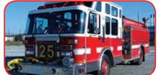
1997 Luverne / Spartan Rescue Pumper Cummins 330 HP, Allison Automatic Hale 1750 GPM Pump Enclosed Pump Panel 1000 Gallon Water Tank AMPS 6KW Hydraulic Generator
