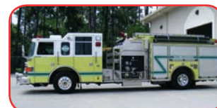
2003 Pierce Enforcer Rescue Pumper Cummins ISL 400 HP, Allison EVS3000P Waterous 2000 GPM Top-Mount Pump 750 Gallon Poly Tank FoamPro 2002 System THREE UNITS AVAILABLE!
