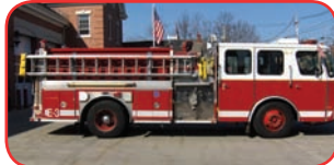
1997 E-One Cyclone Custom Pumper Cummins 300 HP Diesel Engine Allison Automatic Transmission Hale 1500 GPM Side-Mount Pump 750 Gallon Polypropylene Tank
