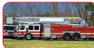
1989 E-One Hurricane 95' Platform Cummins NTC 400 HP, Allison HT740 Hale QSMG 1500 GPM Side-Mount Pump 150 Gallon Aluminum Tank Waterway with Monitor in Platform Onan 6KW Diesel Generator
